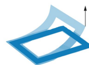
Figure 39: Remove Polyester Frame backing from Incubation Frame
