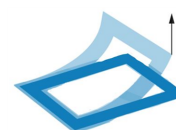
Figure 16: Remove Polyester Frame backing from Incubation Frame
