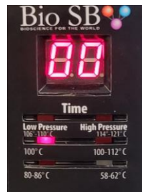
Figure 76: Prime the pressure cooker up to 100° C
