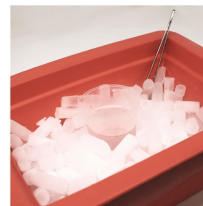
Tissue Freezing & Embedding Isopentane bath setup
